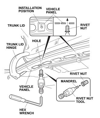
2. Open the trunk. Insert the rivet nut into the hole in the vehicle panel, and install the hex wrench on the rivet nut tool.
